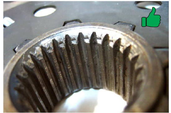
Example of a perfect application amount. This is just enough for smooth installation, and barely visible to the naked eye.
