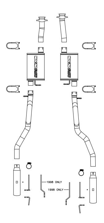
**NOTE:** MAGNAFLOW Performance exhaust systems are designed for a correct fit on vehicles with OEM components. Aftermarket accessories such as headers, and/or cross-over assemblies (H-Pipe / X-Pipe) may not fit like the OEM components, and may require fabrication for proper fit of your MAGNAFLOW system.
