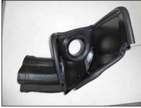
11. Install the provided fresh air duct into the heat shield as shown.
