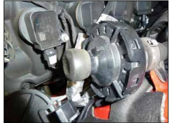
18. Install the provided cap onto the sound drum as shown.
