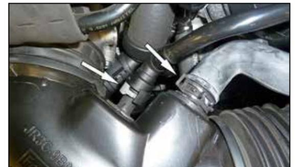
5. Disconnect the vent lines and sound tube attached to the intake tube. Loosen the hose clamps that secure the intake tube to the air filter housing and throttle body and then remove the intake tube from the vehicle.
