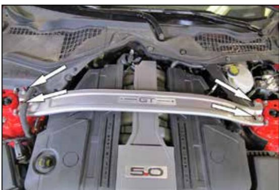
2. Remove the four nuts that secure the strut tower brace and then remove the strut tower brace from the vehicle.
