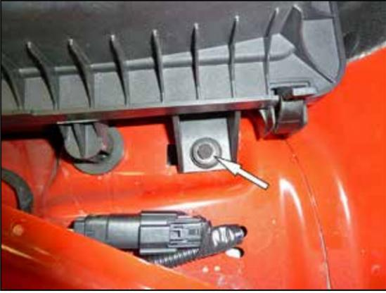
7. Remove the bolt that secures the air filter housing to the inner fender and then remove the lower air filter housing from the vehicle.
