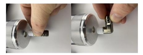
Depending on your application, choose the straight or 90-degree fitting for the base of the catch can and thread it in. Be sure to apply thread sealant tape or paste as needed.
