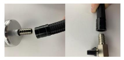
Slide the UPR Billet hose end cover over the end of the hose and push it onto the barbed fitting. Route the hose so that the drain valve would be in a convenient location and trim the hose to length. Install the billet hose end then drain valve, and secure the hose as needed.
