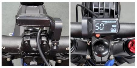
Install the Digital Display onto the bracket with the factory screws. Adjust the positioning to your liking and tighten the bracket. DO NOT OVERTIGHTEN the bracket. The screws just need to be snug enough to secure the bracket. The two bracket halves may not meet depending on the style and model of your handlebars.
