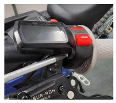
Remove the digital display from the switch assembly by removing 2 screws.
