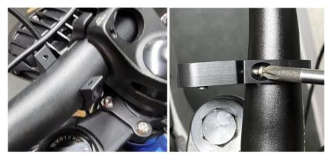
Position the UPR Bracket onto the handle bars and start the screws. DO NOT TIGHTEN the screws at this time.
