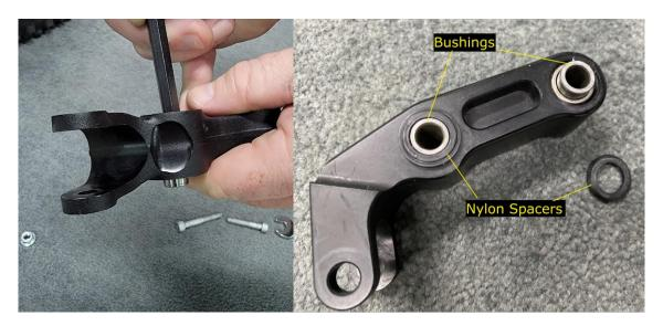
Installation of the new link is the reverse order of removal. Install the new link onto the shock and rotate back into position. Insert the link back into the swing arm then into the triangle link. Do not tighten the hardware until all 3 bolts are installed.
