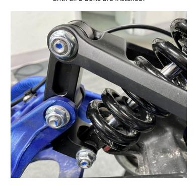
Tighten the fasteners to 18-22 Ft-Lbs /25-30NM
