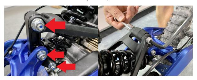
Support the E bike on a stand or lay it on the ground to take weight off of the suspension. Use an 8mm Allen key and a 13mm socket or wrench to remove the 3 fasteners, and remove the stock link. (Some earlier SurRons use a 12mm nut)
