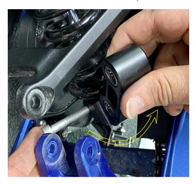
Removing the lower shock bolt is made easier by rotating the shock which will allow the bolt to come out without interfering with the swing arm.
