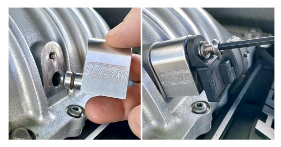
2. Lubricate the O Ring on the UPR Map Sensor Spacer / Adapter with a small amount of oil, then install the spacer with the supplied screw and washer using a 5/32 Allen wrench. Do not overtighten the screw or damage to the sensor and / or supercharger may occur.
