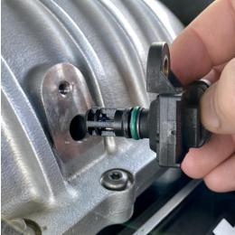
1. Locate the MAP sensor on the driver side of the supercharger. Use a T 27 Torx Bit to remove the screw and remove the MAP sensor from the supercharger. (It is not necessary to un plug the sensor, but you can if you want to)
