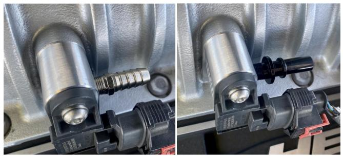
3. The 1/8 NPT port at the back of the spacer can be used to install any type of fitting (not included) for boost reference.
