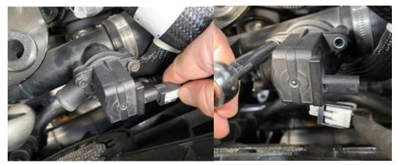
1. Locate the factory blow off valve. Disconnect the wiring harness and remove the 3 attaching screws.
