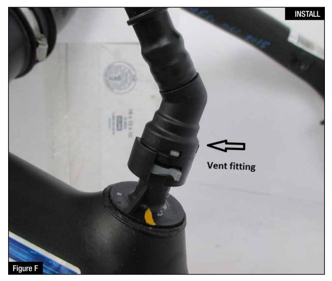
Refer to Figure F for Step 14. (For V6-3.5L (tt) only, not necessary on V6-2.7L (tt) ) Step 14: Locate the valve cover vent tube that feeds into driver's side turbo inlet. It is not necessary to remove the engine cover.
