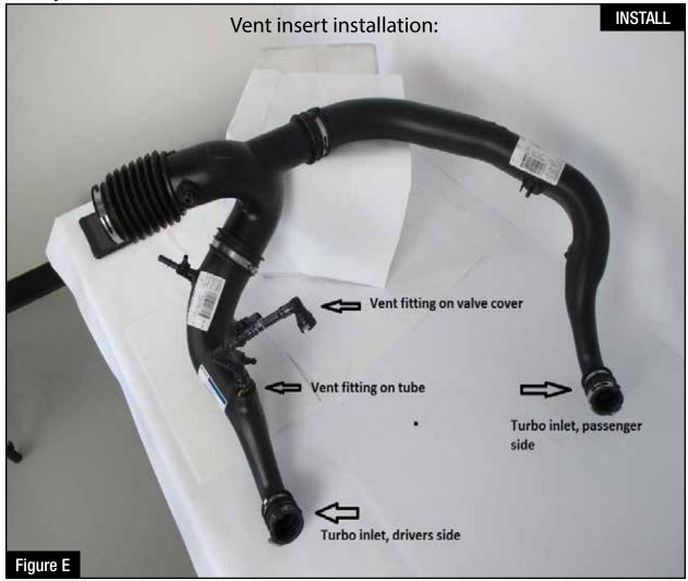
Refer to Figure E for Step 13. (For V6-3.5L (tt) only, not necessary on V6-2.7L (tt) )
