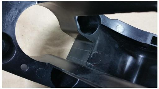
Using a die grinder or dremel tool remove material for adequate pushrod clearance.
