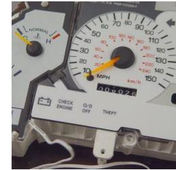
On 1994-1998 Mustangs the left gauge assembly must be removed to install the center overlay. Use a flat screwdriver to pry the gauge assembly out of its sockets. It will simply pop out. Route the overlay electrical wire between the gauge assemblies as pictured, and reinstall the assembly.
