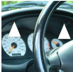
Using a torx screwdriver, remove the two bezel retaining screws from the top of the dash bezel. Once removed, gently pull on the bezel which will pop away from the dash. When the bezel has been removed, remove the four speedo cluster retaining screws. Tilt the cluster outward and detach the two electrical plugs by depressing the tabs on the top. The speedo cluster should now be able to be removed entirely from the dash.
