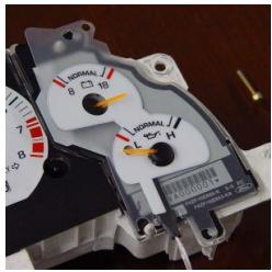
To remove the needles you can use a kitchen fork and evenly pull up on the needle. Be sure to make sure of the position of the needles by using a piece of tape and mark the numbers it was pointing at or a black marker stripe on the side of the housing. Repeat the same procedure for each piece. For 1999+ Mustangs the gauge set is one piece, but the same procedure applies.
