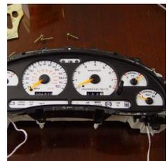
Re-install the black / clear bezel and the gold retaining screws.
