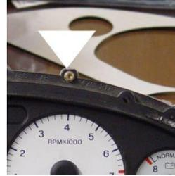
Once the speedo cluster is removed from the car, place it on a desk or flat surface to begin the silver Faced reverse gauge installation. Remove all of the gold colored retaining screws that surround the outside of the clear / black plastic housing. The black bezel and clear plastic should now be able to separate from the cluster.
