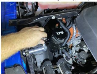
3. Remove the Factory PCV hose. It connects from the passenger side valve cover fitting to the supercharger vacuum fitting.
