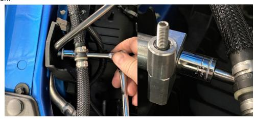
2. Install the UPR One Way Breather catch can using the supplied quick release knob.
