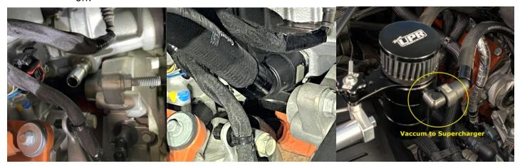
5. The 'Dirty Side' Hose will have 90 degree fittings on one end. Connect the 90 degree end to the valve cover fitting, and the 45 degree end to the rear fitting on the catch can.
