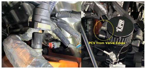
The catch can, filter, and components can be washed with warm water and mild detergent like dish soap or Simple Green as needed. UPR does not recommend using solvent based cleaners.
