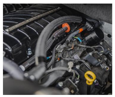
6. If you selected to add the Clean Side Separator, remove the driver side crankcase vent hose. It will connect from the driver side valve cover to the air box or cold air intake. Install the Clean Side Separator by lifting the collar at the base and pushing it onto the male fitting on the valve cover. It will snap into place when it is seated. Install the provided hose as shown.
