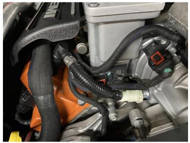
1. Locate the factory PCV hose that runs from the passenger side valve cover PCV fitting to the supercharger vacuum fitting and remove it. Save this hose in case you ever want to return the vehicle back to stock.
