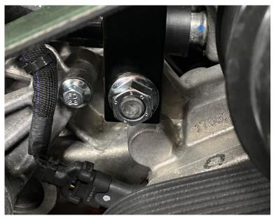
2. Mount the catch can bracket to the stud on the passenger side of the water pump with the supplied nut.
