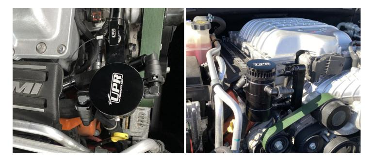
4. Mount the catch can to the bracket. Connect the PCV side hose to the front facing fittin of the catch can by running the hose under the bracket as shown. Connect the remaining hose that is connected to the supercharger vacuum fitting to the other side of the catch can.
