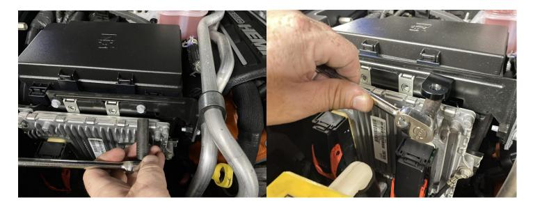
2. Use a 10mm wrench or socket to remove the right side bolt from the ECU mount. Install the UPR 90-degree billet bracket as shown using the supplied bolt.
