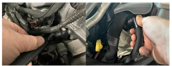
4. Install the hoses onto the engine by pushing the UPR Plug N Play<sup>™</sup> female fittings onto the vacuum and PCV male fittings until they click.
