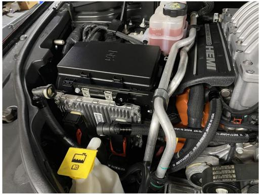
3. The longer of the two hoses in the kit will be the PCV or 'dirty' side hose. The vacuum hose, or 'clean' side hose will be shorter. Route the hoses behind the AC lines as shown. If you selected to add a UPR Check Valve to your catch can kit, it will be installed in the 'clean' hose when the kit is built. Be sure the arrows on the check valve are facing towards the engine when routing the hose.
