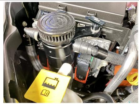
5. Install the UPR catch can onto the 90-degree billet bracket with the supplied bolt. Install the UPR Plug N Play<sup>™</sup> Fittings onto the catch can. The 'Dirty' side hose will connect to the left side of the catch can. The 'clean' side hose will connect to the right side of the catch can.
