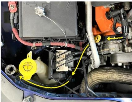
5. Install the clean side hose to the supercharger snout. Make sure arrow on check valve is facing away from the catch can. Route the clean side hose above the alternator and tensioner, between the ABS system and the fuse panel, to the fender mount as pictured.
