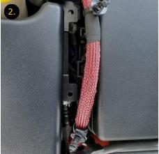
**3.** Locate the Factory PCV hose that runs from the passenger valve cover to the Vacuum fitting on the supercharger and remove it.
