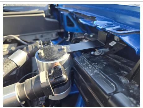
**3B**. For Mavericks not equipped with LED headlights, the headlight assembly will be too long and will interfere with the spacer. For these vehicles remove the 2 screws on the top of the catch can and flip the bracket over. Reinstall the screws. Install the catch can bracket onto the fender bolt with the nut from the spacer.
