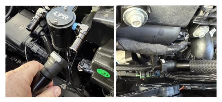
4. The clean side of the catch can will be marked with a silver ring at the end of the male fitting. Connect the shorter hose from the catch can to the intake manifold vacuum fitting. The 45 degree fitting will go to the intake manifold, the straight fitting will connect to the catch can.
