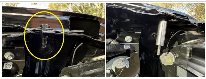
2. The catch can will mount off the fender bolt on the driver side close to the headlight. Screw the provided aluminum stud assembly onto the bottom of the fender bolt, and tighten it using the allen wrench. \*For Mavericks not equipped with LED headlights, see step 3B
