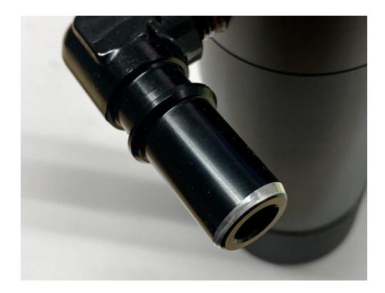
**6.** The outlet fitting on the catch can that will connect to the vacuum hose will have a silver marking at the end of the fitting as shown.
