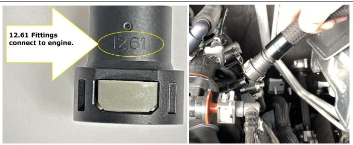
**5.** Connect the other hose to the intake manifold vacuum fitting using the hose end with '12.61' printed on it.
