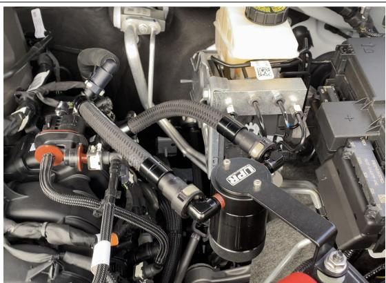
To service the catch can, unscrew the catch can cup and dispose of the contents with used waste oil according to your local laws.
