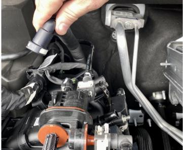
3. Move the PCV hose to the other side of the EVAP hose by routing it under the EVAP hose as shown. This will help to stabilize the hose when connected to the catch can.
