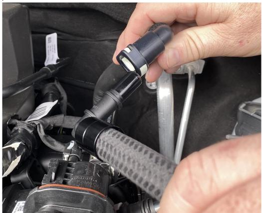
**4.** Connect the hose with the male 90 degree fitting to the factory PCV hose.
