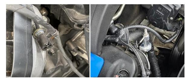
3. Install the UPR catch can onto the billet bracket with the supplied hardware.
