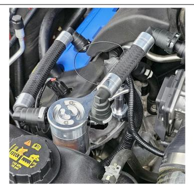
4. The inlet side of the catch can will be closer to the cylinder head, while the outlet will be closer to the intake manifold. The longer hose in the catch can kit will be the PCV hose. It will connect from the PCV fitting on the passenger side valve cover to the inlet side of the catch can. The other hose will connect from the outlet to the intake manifold vacuum fitting.
