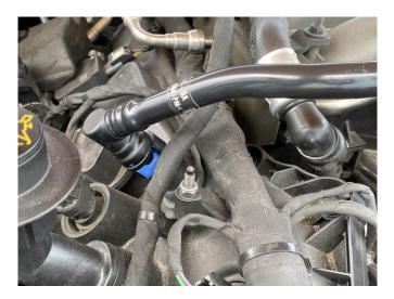
2. Locate the grounding stud on the front of the passenger side cylinder head. Remove the protective cap and install the L shaped bracket.
