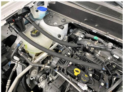
**9.** Once you remove the factory CCV tube, connect the hoses as shown. Straight fittings go to the catch can. 90 degree fitting goes to the valve cover, and the 45 degree fitting goes to the air intake tube.
