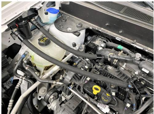
**8.** Once you remove the factory CCV tube, connect the hoses as shown. Straight fittings go to the catch can. 90 degree fitting goes to the valve cover, and the 45 degree fitting goes to the air intake tube.
