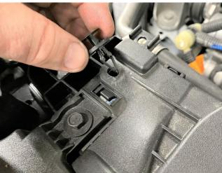
**1.** Remove the 2 fasteners from the air inlet duct. A flat screwdriver works well. Lift the center of the fastener, then the fastener body. Lift up and remove the air inlet duct.
