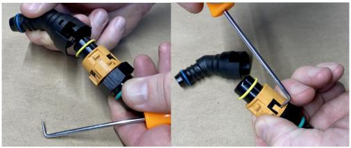
Now that you can see the 3 retainer tangs, while applying upward pressure, use a pick or small screwdriver to release them.
