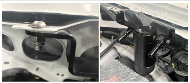
**3.** Using the supplied hardware, install the catch can onto the driver side fender tab. The catch can bracket will face forward to avoid interference with the hood. If needed, you can bend the bracket up slightly to gain clearance between the catch can and fuse box.
