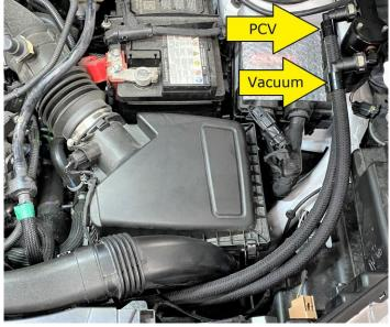
**5.** Connect the PCV hose. The PCV valve will swivel slightly which may make connecting the hose a little more difficult. Once the UPR Plug N Play fitting is fully engaged, it will click. Route the hoses along the front side of the intake air box inlet duct connection towards the catch can. You can secure the hoses to the engine cooling fan wiring harness (arrow) with a zip tie if you like. Reinstall the air intake duct once you are happy with the hose routing.
