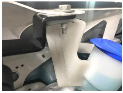
7. The Clean Side Catch Can will mount on the passenger fender using the factory washer bottle nozzle bolt. Remove the bolt, slide the catch can bracket between the tab and washer bottle mount, then reinstall the bolt. The catch can bracket will face forward to avoid interference with the hood.
