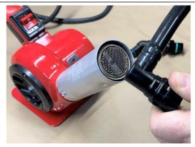
To replace the fittings on your factory CCV tube, use a heat gun or lighter to gently warm the plastic tube – do not melt or burn the tube. Pull the fitting out of the tube once it is warm, (Careful, it will be hot) and insert the new fitting into the tube while it is still warm. The tube will conform to the fitting as it cools. To assist, you can wrap a small zip tie around the tube ends.
