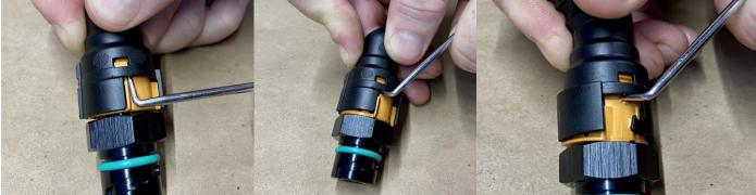
**7.** Locate the Crankcase Vent Tube on the valve cover towards the passenger side of the engine. The Tube will have 2 orange fittings that are not a quick release style fitting.
