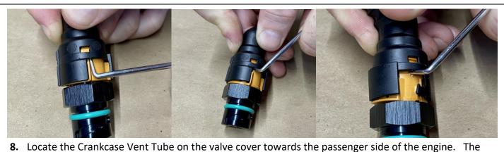
Tube will have 2 orange fittings that are not a quick release style fitting.
