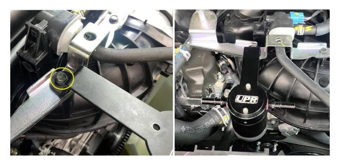
1. Remove the engine cover (if equipped) by lifting it up and pulling it towards the front of the truck. Locate the bolt on the left side of the front engine cover mount. Use a 10mm socket to remove the bolt, position the bracket so it points towards front of the truck, bolt it down reusing the stock bolt.
