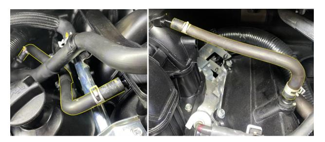
2. Locate the PCV hoses on the driver and passenger side of the engine. The hoses will run from the valve covers to the intake manifold. Use a pair of pliers to squeeze the clamps and move the clamps away from the end of the hoses. Remove the hoses. Keep them in case you ever want to return the truck back to stock.
