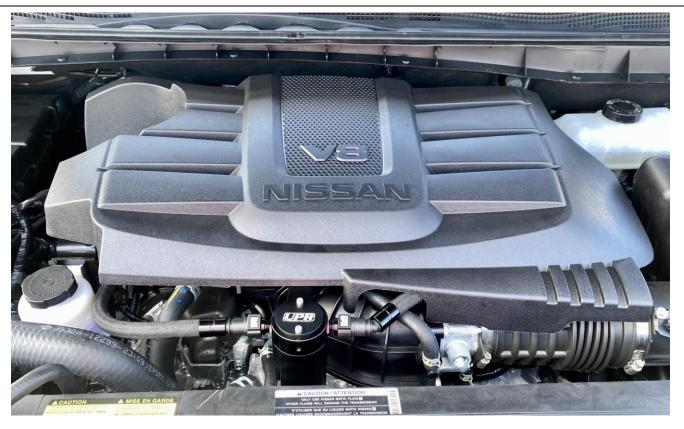
5. Go back over all of the connections to make sure the hoses are routed neatly and away from any hazards. Reinstall the engine cover.
