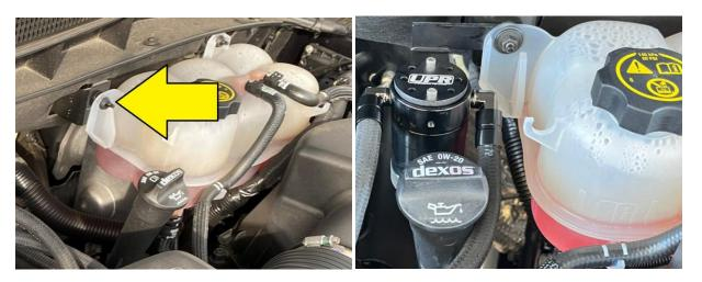
2. The catch can will mount to the coolant reservoir stud with the supplied hardware.
