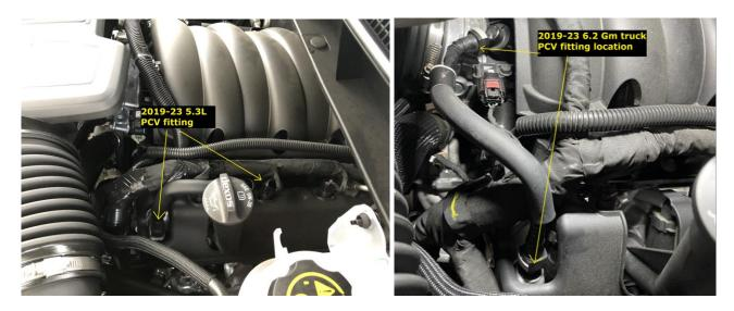
1. Locate the PCV hose on your truck. The hose on **5.3** liter engines will run from the PCV fitting on the driver side valve cover to the intake manifold vacuum fitting on the side of the intake manifold.
