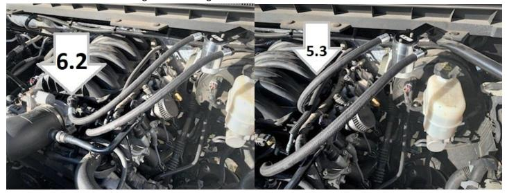
4. Connect the other hose to the Vacuum port on the intake with the UPR Plug N Play ™ fitting, and connect the other end of the hose to the remaining barbed fitting. Go back to check the connections to make sure they are secure. That's it, all done!
