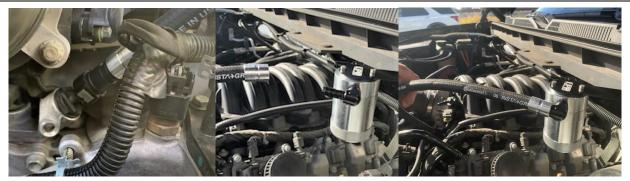
3. Connect the UPR Plug N Play ™ fitting to the factory PCV fitting. The Plug N Play ™ fitting Will click on when fully seated. Slide the UPR billet hose end onto the hose and push it all the way onto the forward-facing barbed fitting on the catch can.
