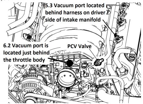
2. Locate the factory PCV hose and remove it. The 5.3 PCV hose will run from the PCV in the lifter valley plate to the vacuum port on the driver side of the intake manifold about half way down. The 6.2 will have a short hose from the PCV in the lifter valley plate to the top of the intake manifold just behind the throttle body.
