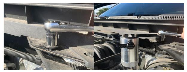
1. Use a 13mm socket or wrench to remove the fender support bolt at the cowl on the driver side of the engine compartment. Use the same bolt to install the UPR catch can bracket onto the support.
