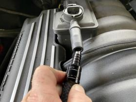
**3.** The vacuum boot will push directly onto the catch can fitting on the right side of the catch can. Install the barbed fitting and the billet hose end onto the catch can PCV hose. Push the fitting into the PCV boot.
