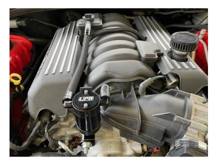
**4.** Double check the connections to make sure they are secure. Be sure the catch can mount is tight, and the containment cup is secure. Check the containment cup every 500 miles at first to get to know your engine's needs. To empty the catch can, the cup is unscrewed from the catch can body. Always dispose of the liquid with used oil according to local laws. Do not over tighten the catch can cup, it just needs to be snug.
