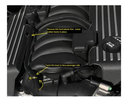
1. Remove the factory plastic PCV tube. Leave factory rubber PCV boots in place. Twist the 90-degree boot to face the front of the engine.
