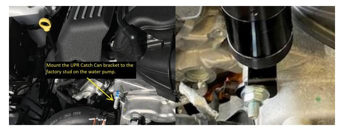
2. Using the supplied hardware, mount the UPR catch can bracket to the factory stud on the water pump as shown.
