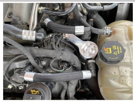
4. The inlet side of the catch can will be closer to the cylinder head, while the outlet will be closer to the intake manifold. The longer hose in the catch can kit will be the PCV hose. It will connect from the PCV fitting on the passenger side valve cover to the inlet side of the catch can. The other hose will connect from the outlet to the intake manifold vacuum fitting.
