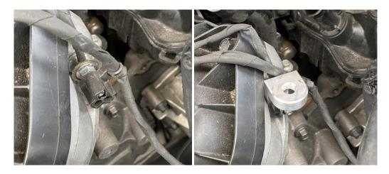
3. Install the UPR catch can onto the billet bracket with the supplied hardware.
