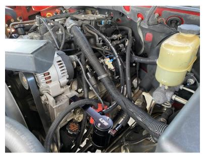
Always check and drain the catch can more often in winter / freezing weather. If the water/oil mixture in the catch can is allowed to freeze it will cause damage to the catch can and internal components. Any damage due to freezing is NOT WARRANTY. You must dispose of the liquid collected in the catch can properly (with used waste oil) properly according to your local laws.
