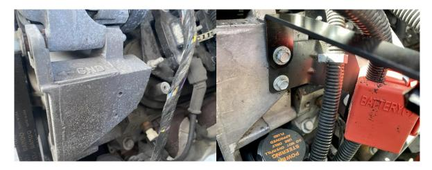
2. Locate the factory PCV tube. It will run from the PCV or PCV fitting at the back of the driver side valve cover to the top of the intake manifold.
