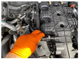
**6.** The UPR catch can kit will include 2 hoses. One will have a 45-degree fitting, and the other will have a 90-degree fitting. Install the hose with the 45-degree fitting onto the intake manifold vacuum port, and the hose with the 90-degree fitting will install onto the PCV valve.
