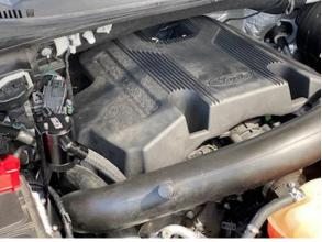
Check the catch can every 500-1000 miles to get an idea as to your engine's needs. Do not let the catch can overfill. All catch can components can be cleaned with warm water and mild detergent like dish soap. UPR does not recommend the use of solvents or harsh chemicals as they can damage the finish and O rings.
