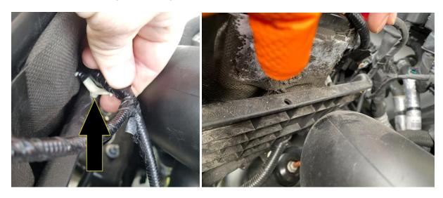
2. Using the retainer hole as a starting point, and the bracket as a template, mark the location to drill a second 1/8" starter hole for the bracket retaining hardware. NOTE\* on some year and model trucks, you may need to relocate the bracket slightly depending on the location of the support ribs on the battery tray. Check to make sure the ribs will not be in the way before drilling or attempting to install hardware.
