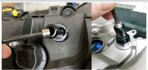
Once you have selected the size restrictor jet to use, it simply threads into the PCV fitting using the supplied Allen wrench.
