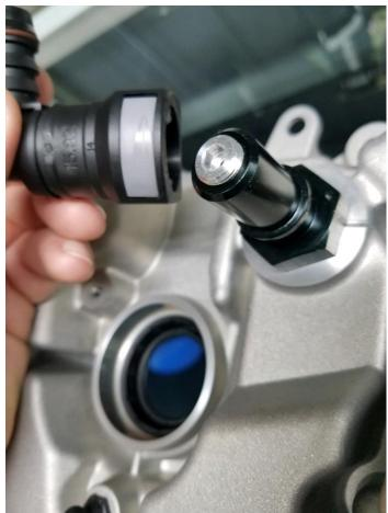
The Restrictor Jet will protrude slightly from the end of the fitting. The factory or UPR Plug and Play fitting can now be reinstalled.
