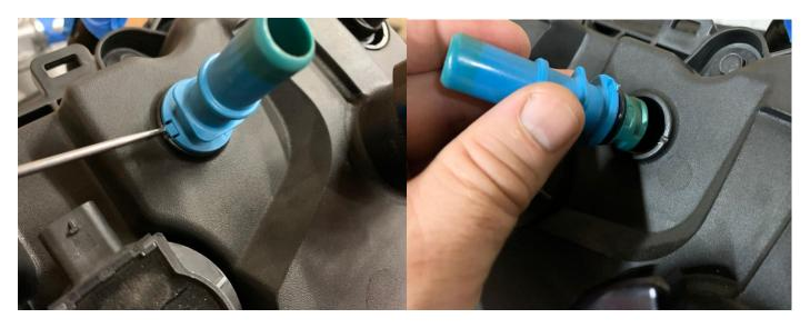
Remove the factory PCV valve by gently lifting the tabs on either side with a small screwdriver or pick, and unscrew the fitting. It is a ¼ turn fitting and should come out by hand.
