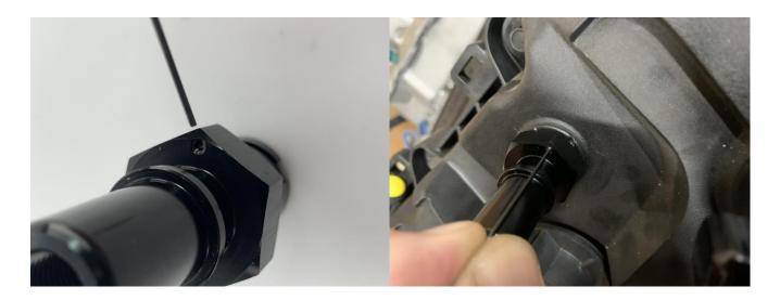
UPR Billet valve cover fittings have a pair of small Allen head set screws in the base. The set screws are designed to be tightened until the base of the screw comes into contact with the valve cover. This keeps the fitting from rocking and rotating in the valve cover. The set screw locations will not necessarily meet the valve cover in the same spot as the factory tangs.
