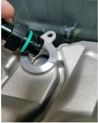
Align the fitting with the tangs in the valve cover. The fitting will work with factory style Plastic or Aluminum valve covers. **CAUTION** with Plastic valve covers- install the Billet fitting **BY HAND** as the plastic tangs will be damaged by overtightening.
