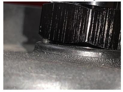
**DO NOT OVER-TIGHTEN** the set screw as it can damage the fitting or valve cover.
