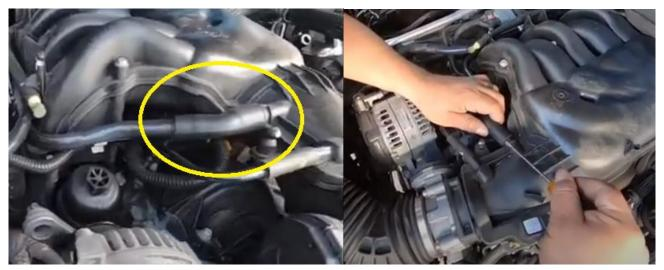
2. Remove the intake cover and locate the PCV tube. Remove the rubber boot (circled) from the intake manifold vacuum port. The rubber boot can become stuck, so you may need to use a small screwdriver or pick to separate it.
