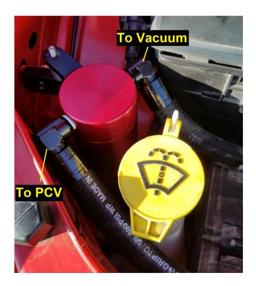
Always check and drain the catch can more often in winter / freezing weather. If the water/oil mixture in the catch can is allowed to freeze it will cause damage to the catch can and internal components. Any damage due to freezing is NOT WARRANTY. You must dispose of the liquid collected in the catch can properly (with used waste oil) properly according to your local laws.
