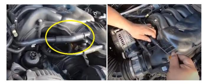
4. Locate the PCV tube. Remove the rubber boot (circled) from the intake manifold vacuum port. The rubber boot can become stuck, so you may need to use a small screwdriver or pick to separate it.
