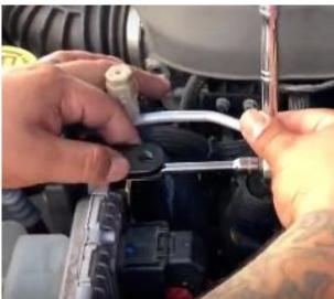
1. Locate the ECU which is on the driver side of the engine compartment. Using an 8mm socket, remove the factory mounting bolt on the top ECU mount that is closest to the engine. Using the supplied bolt, install the UPR billet L bracket onto the ECU mount.
