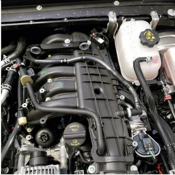
3. Remove PCV line from driver side of engine behind TB (Push Button on fitting to release)
