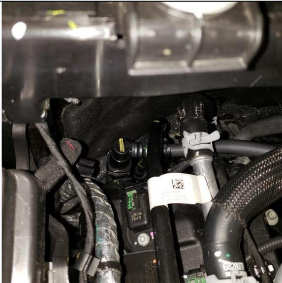
2. Remove PCV line from passenger side rear of engine (Push Button on fitting to release)
