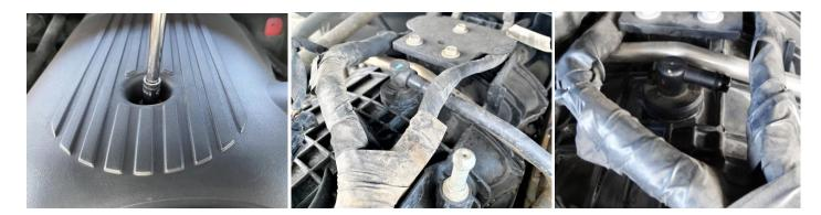
2. To remove the hose you can cut it lengthwise along the plastic fitting and spread it apart, exposing the barbed fitting, or cut out a section of hose so you can slip the UPR hose over it.
