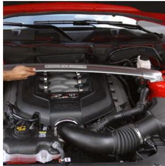
Remove the strut tower brace.
