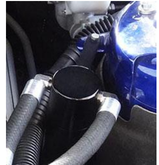
Drill a 5/16 hole in the tab just off of the driver side strut tower. Secure the catch can with the provided 5/16 bolt and nut.
