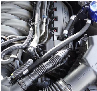
Connect the inlet side of the can to the valve cover and the outlet side to the intake tube using the provided Ford OEM fittings.
