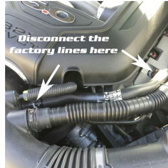
Disconnect the factory PCV line from the valve cover to the intake tube.
