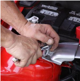
Remove the (4) 13mm nuts holding the strut tower brace in place if equipped.
