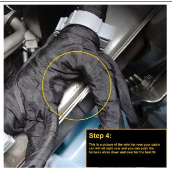
This is a picture of the wire harness your catch can will sit right over and you can push the harness wires down and over for the fit best fit.
