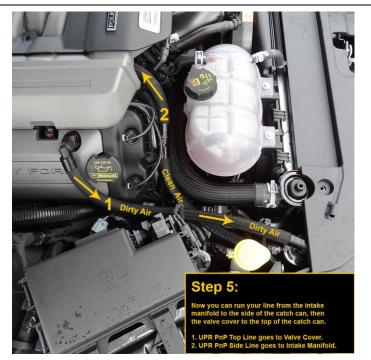
Now you can run your line from the intake manifold to the side of the catch can, then the valve cover to the top of the catch can.
