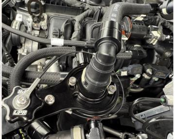
**4.** Connect the hose with the male 90 degree fitting to the factory PCV hose, then connect the other end to the top fitting on the catch can.
