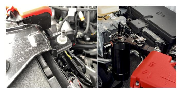
1. The UPR catch can will mount to the battery hold down stud using the supplied nut. Install the nut to retain the catch can bracket, and tighten the nut with a 13mm wrench.
