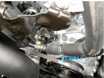
7. Locate the Crankcase vent tube. It has an orange fitting on the front part of the valve cover and connects to the turbo inlet tube. These fittings are not quick release style, and the best way we have found to remove them is to use a pick to disassemble the fittings on the vehicle.
