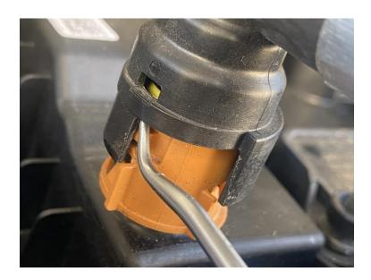
**8.** Use a curved or 90 degree pick to pry the outer black part of the fitting off of the orange inner part. Insert the pick just below the small orange rectangular 'window' and pry up. Repeat this on the other side of the fitting.
