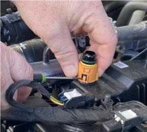
**9.** Now that you can see the 3 tangs, while applying upward pressure, use a pick or small screwdriver to release them and remove the rest of the fitting from the valve cover.
