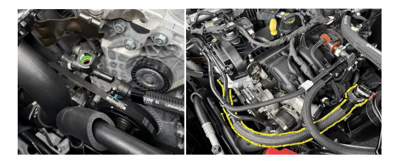
**10.** Install the 3 way fitting onto the Turbo Inlet tube. Be sure the male portion of the fitting is facing towards the driver side. Connect the 45 degree fitting on the WOT hose to the male portion of the fitting, then connect the 90 degree end to the catch can. The arrow on the check valve in this hose will face away from the catch can.
