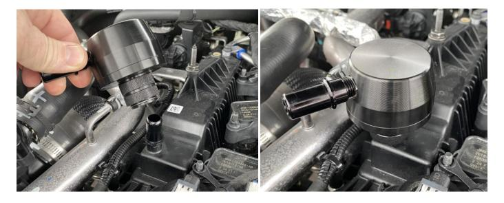
**11.** To install the Clean Side Separator (CSS) pull up on the collar at the base of the CSS and push it down onto the CCV fitting on the valve cover. Once the CSS is installed fully onto the CCV fitting, the collar will click on to secure it.
