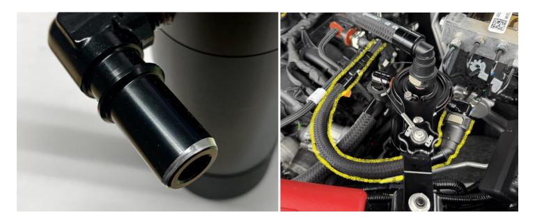
**6.** The outlet fitting on the catch can that will connect to the vacuum hose will have a silver marking at the end of the fitting as shown. Connect the vacuum hose to the catch can fitting closest to the driver side fender. Wrapping the hose around the catch can in this manner will reduce the chances of kinking the hose.
