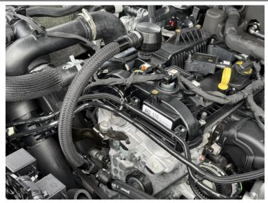
12. Install the last hose from the Clean Side Separator to the 3 way fitting.
