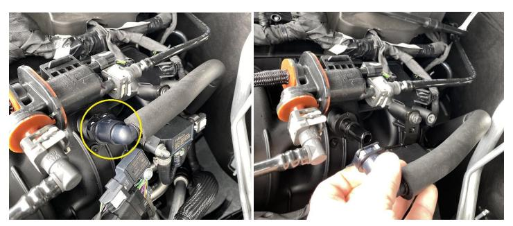
2. Locate the PCV hose on the intake manifold on the driver side of the engine (circled). Release the fitting by pressing the button at the bottom of the fitting (do not pry the button out) and slide the hose off of the intake manifold.
