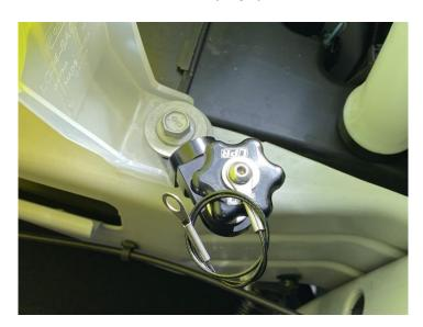
2. Install the UPR catch can bracket with the provided 8mm bolt. (factory bolt will also work) Leave this bolt a little loose so you can adjust the catch can position.
