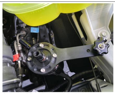
3. Use the 10mm UPR knob to install the catch can onto the bracket.
