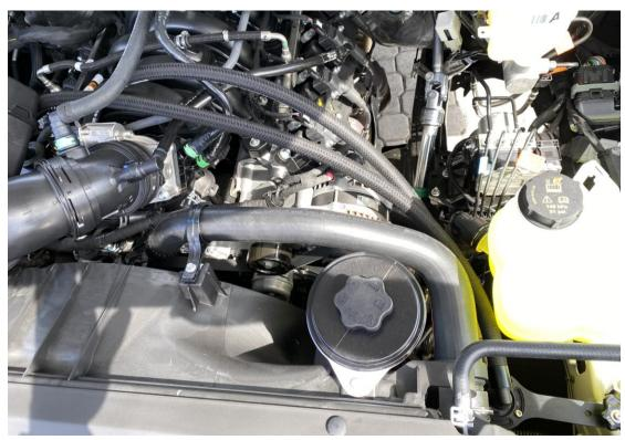
7. Once you are satisfied with the routing of the hoses, go back and tighten the catch can bracket bolt and knob.
