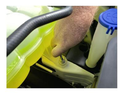
1. Use a 13mm socket to remove the factory bolt holding the Coolant Degas Bottle to the driver side front frame rail.
