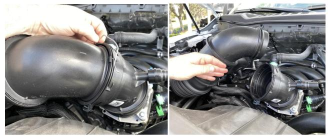
4. To help gain access to the PCV hose, you can remove the clip from the air intake tube and pick it up.
