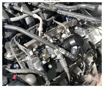
8. Install the the CSS, be sure the collar on the bottom is pulled up, it will snap when seated onto the fitting. Rotate the factory crankcase vent fitting in the hose and connect it to the CSS.
