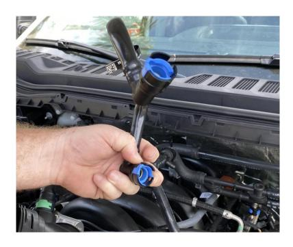
5. Locate the factory PCV hose that connects from the PCV valve on the passenger side valve cover to the intake manifold vacuum fitting.
