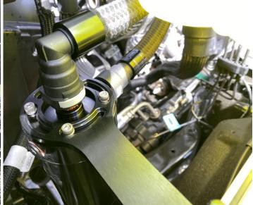
6. The Vacuum hose will have a 90 degree fitting and a 45 degree fitting. Connect the 90 degree fitting to the intake manifold vacuum port, and the 45 degree fitting to the side fitting on the catch can. The PCV hose will have 90 degree fittings on both ends. Connect the hose from the PCV valve to the top fitting on the catch can. Be sure to route the hoses away from any hazards like pulleys or fans.
