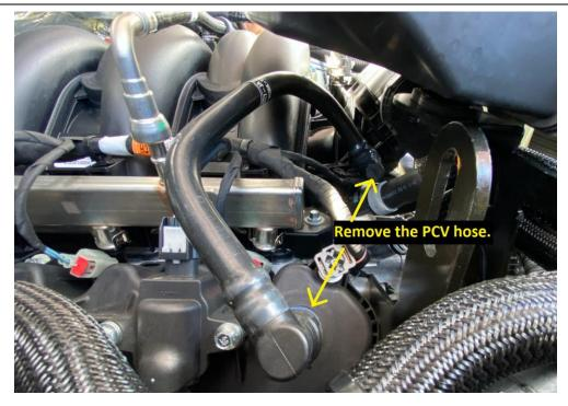
The fittings are removed by pushing the retainer to the side and lifting the fitting off.
