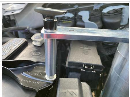
Install Threaded stud onto battery hold down stud and tighten. Install Catch Can with knob.
