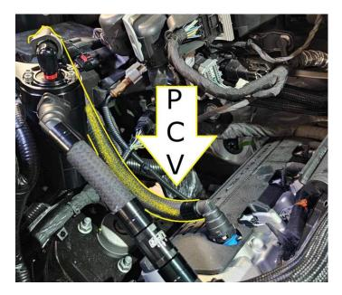
**4.** Connect the 'Dirty side' hose with the 90 degree fittings to the PCV value on the value cover. The other end of the hose will connect to the top fitting on the catch can. The hose should run down along the value cover, then up to the catch can fitting as shown in the pictures below.
