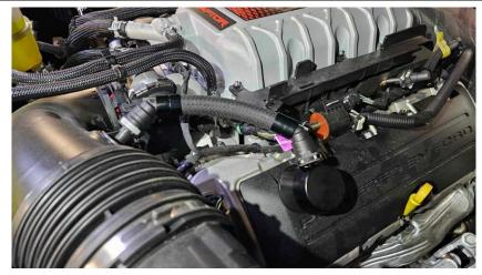
**7.** Install the CSS with the supplied hose assembly. When installing the CSS, be sure the collar on the bottom is pulled up, it will snap when seated onto the fitting.
