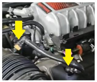
**6.** To install the Clean Side Separator (CSS), you will need to remove the orange fittings on the driver side Crankcase vent hose. These fittings are not a quick release style.
