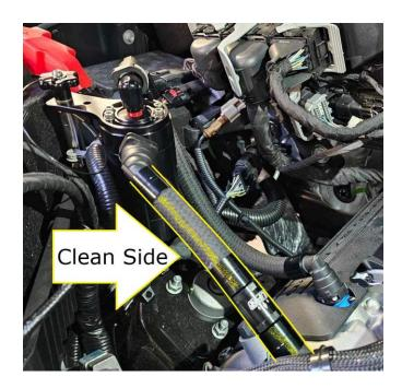
3. The 'Clean side' of the catch can will be the fitting on the side of the can. Connect the hose with the 45-degree fitting on the can, and connect the straight end to the vacuum port on the supercharger. \* If you selected to add the check valve to your kit, the arrow on the check valve in this hose will face away from the catch can, towards the engine.
