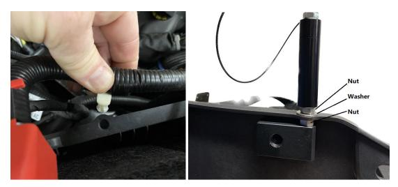
2. Locate the factory PCV hose that runs from the passenger valve cover PCV valve to the Supercharger vacuum port. Remove the factory fittings by pushing the blue tabs on the fittings to the side and lift the hose off.
