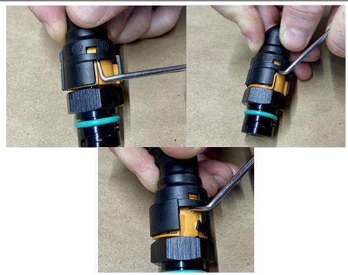
Now that you can see the 3 tangs, while applying upward pressure, use a pick or small screwdriver to release them.
