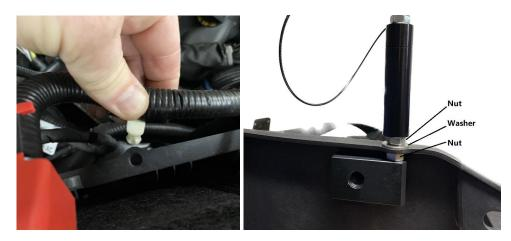
**B\* Optional Step.** To increase the stability of the mount, start by marking the location of the hole in the support block, drill a 3/8 hole (this is best done with the battery removed) and install a 3/8-24 bolt from the inside of the battery tray out through the bracket. You will need to cut a small portion of the inner support ribs to make room for the bolt.
