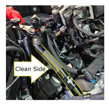
**3.** The 'Clean side' of the catch can will be the fitting on the side of the can. Connect the hose with the 45-degree fitting on the can, and connect the straight end to the vacuum port on the supercharger. \*
