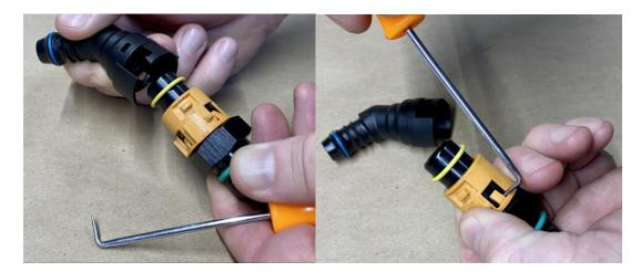
If you want to return your vehicle back to stock, you can replace the fittings on the driver side hose with UPR part number 2025-39 and 2025-40. Use a heat gun or lighter to gently warm the plastic tube – do not melt or burn the tube. Pull the fitting out of the tube once it is warm, and insert the new
