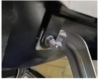
13. Remove the 10MM nut on the ABS brake controller bracket. Install the UPR Clean Side Catch Can bracket and reinstall the nut. You may bend the bracket slightly to allow the catch can to sit level.
