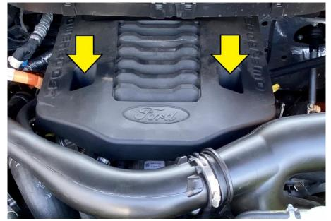
3. Remove the engine cover to gain access to the PCV fittings. It will have two 10MM nuts holding the cover on. Use a 10mm deep socket and extension to remove them, then lift the cover off.
