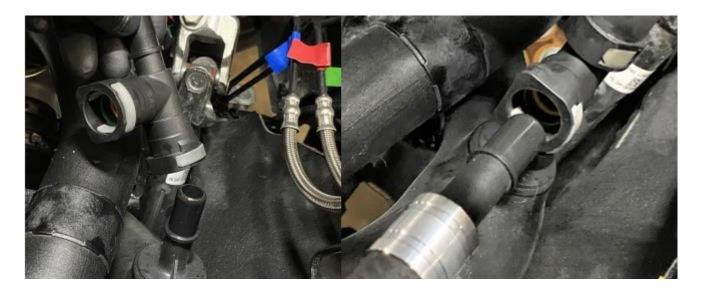
12. Install the 3-way Plug N Play Wide Open Throttle adapter fitting onto the driver side turbo inlet tube so that the female leg of the Tee is facing forward. Route the last hose (the Wide Open Throttle or WOT hose) from the catch can to 3 way fitting. Connect the male fitting on the WOT hose from the catch can to the female fitting on the Tee.
