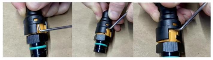
9. Another Method to remove the fitting is to separate the orange portion of the fitting from the outer cover. Using a pick or flat screwdriver, find the small orange 'window' on each side of the fitting. Slide the pick or screwdriver up between the black outer portion of the fitting and the orange inner portion. Pry up on each side to pop the outer portion off.
