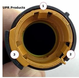
7. Use a 90-degree pick or hook pick to release the fitting. There are 3 little tabs securing the female end of the fitting onto the valve cover fitting.
