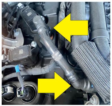
4. Locate the factory PCV tube on the passenger side of the engine. It runs from the PCV valve on the valve cover to the intake manifold vacuum port. Remove the tube by releasing the factory fittings.
