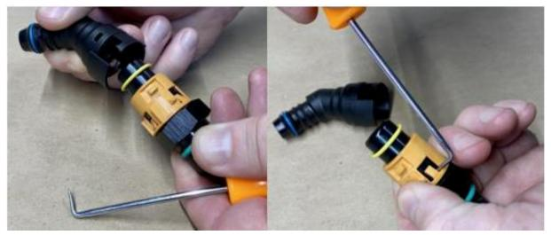
10. Now that you can see the 3 tangs, while applying upward pressure, use a pick or small screwdriver to release them.
