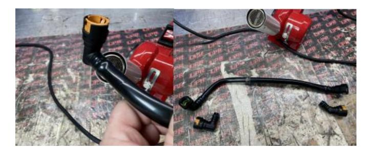
11. To replace the fittings on your factory CCV tube, use a heat gun or lighter to gently warm the plastic tube – do not melt or burn the tube. Pull the fitting out of the tube once it is warm, (Be careful, it will be HOT) and insert the new fitting into the tube while it is still warm. The tube will conform to the fitting as it cools. To assist, you can wrap a small zip tie around the tube ends while it cools.
