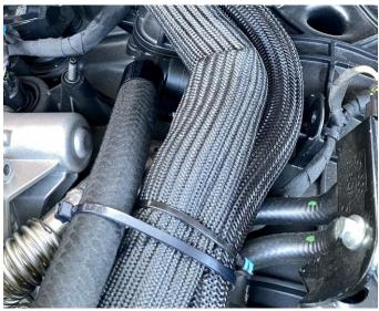
15. Secure the hoses to ensure they do not encounter any hazards like hot components, fans or belts. A good tip is to zip tie the vacuum hose along the coolant hoses on top of the intake manifold.
