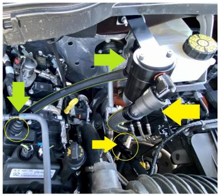
14. Install the longer of the 2 hoses onto the driver side valve cover fitting, and connect it to the rear fitting on the catch can. Connect the front fitting of the catch can to the top of the 3 way fitting on the turbo inlet tube.
