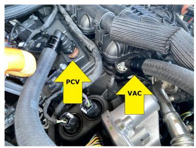
5. Time to start routing hoses. Connect the hose with **no check valve** in it to the passenger side valve cover PCV valve and route it to the catch can center inlet port. Be sure to route hoses so they will not contact any belts, pulleys or other hazards.
