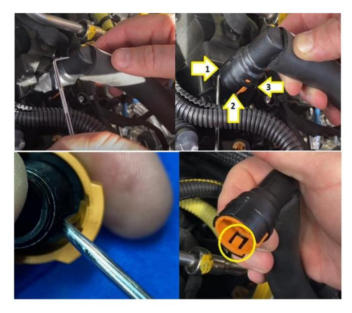
8. While holding the hose and applying slight upward pressure, run the pick under the fitting to release the tabs. If the fitting or tabs break, the fitting can be replaced with a standard UPR Plug and Play fittings P/N 2025-39 (straight), 2025-40 (90 degree) or 2025-41 (45 degree). Repeat the process to remove the fitting at the other end of the tube.
