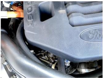
16. Reinstall the engine cover and tighten the 10mm nuts. Be sure the hoses clear the cover and do not interfere with other engine components.
