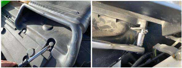
2. Locate the Square hole to the rear of the oval shaped hole on the flat portion of the frame on the driver side directly below the air inlet. Install the 90 degree mounting bracket to the frame with the supplied hardware as shown. The bracket should be facing upwards. Install the catch can onto the bracket with the supplied hardware. You can adjust the angle of the catch can by loosening the screws on the can and clock it into the best position.
