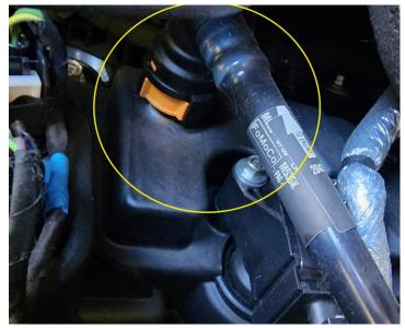
6. On the 2021-up 3.5L Ecoboost F150s, the driver side CCV (Crankcase Vent) hose is secured with special orange fittings. There is no tool available through Ford to remove this fitting. To Install the Clean side catch can, and WOT (Wide Open Throttle hose) you will need to remove these fittings.
