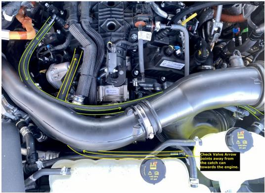
Find the longest hose in the kit with a check valve in it. Route the hose so that the arrow printed on the check valve faces away from the catch can, towards the engine. Connect the hose to the intake manifold vacuum port, and the other end to the outlet port that is furthest forward on the catch can. We found it easiest to route the PCV hose along the intake tubes going to the air box, and the vacuum hose forward and along the coolant bottle.
