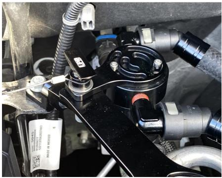
**1.** If you selected the clean side catch can: Attach the clean side catch can bracket to the PCV side catch can bracket with the same knob used to install he PCV catch can.
