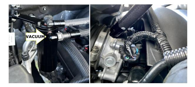
**3.** Install the 'Clean Side' hose to the side fitting on the catch can, and connect it to the vacuum port just behind the throttle body ( if you selected to add the Billet Pro Series check valve, the arrow faces away from the catch can, towards the engine)
