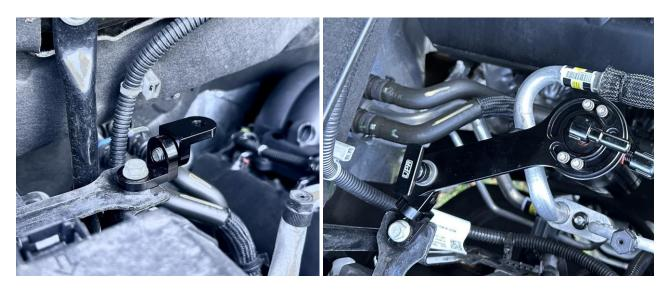
1. Remove the battery hold down bolt, then install your UPR Catch Can bracket in this location re using the factory bolt. Position the catch can so that it does not interfere with any of the AC lines and tighten the bolt.
