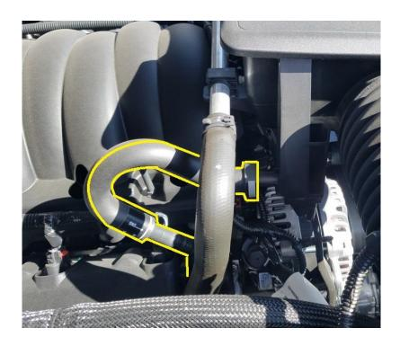
**2.** Remove the clean side hose from the passenger side of the engine. Press the buttons on the fittings to release them.
