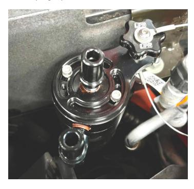
2. Attach the catch can to the UPR billet bracket with the supplied knob. You can leave the catch can slightly loose to allow adjustment when routing hoses. The allen screws at the top of the catch can allow for adjustment as well. Once the hoses are routed, adjust the catch can for best fit and tighten fasteners.
