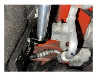
1. Using the supplied hardware, attach the UPR billet catch can mounting bracket to right side hole at the front of the battery tray. To make this easier, you can remove the battery hold down bracket which will allow you to move the battery slightly
