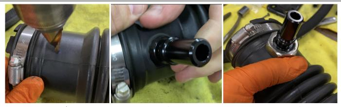
7. Use a 5/8 or 16mm drill bit to make a hole for the UPR Plug and Play™ Quick tap Fitting. (A step-drill bit works well). Install the fitting from the inside-out. Use the washer, retaining nut and clip to secure it. DO NOT OVERTIGHTEN the fitting or it can crack the tube. If you drilled the hole a little too big, don't panic. You can use a dab of automotive silicone sealant on the quick tap fitting.
