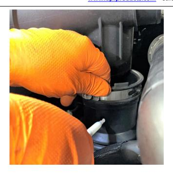
5. The third hose is the Wide Open Throttle hose (WOT). It will have straight fittings on each end and a check valve in it. Connect the hose to the catch can and route it towards the passenger side turbo inlet tube. It is the lower rubber tube connected to the air box. Be sure the Arrow printed on the check valve faces away from the catch can. Mark the tube where the hose will comfortably reach. This is where you will install the UPR Quick Tap fitting.
