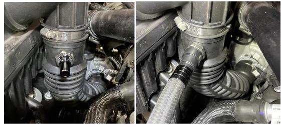
8. Reinstall the air inlet tube, and connect the WOT hose connector.
