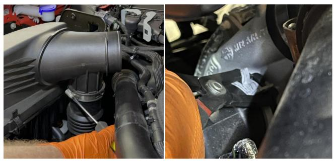
6. After marking the tube, remove the passenger side turbo inlet tube by loosening the hose clamps at the air box, and remove the air box cover. Use a pair of pliers to squeeze the clamp on the turbo inlet. When squeezed all the way, this clamp is designed to lock open which will aid re assembly.
