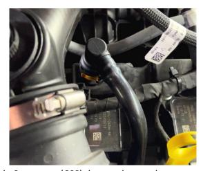
9. To install the Clean Side Separator (CSS), locate the crankcase vent fitting on the driver side valve cover.
