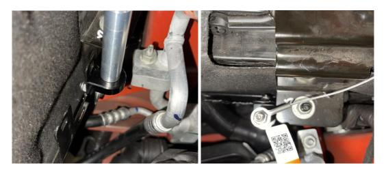
1. Using the supplied hardware, attach the UPR billet catch can mounting bracket to right side hole at the front of the battery tray. To make this easier, you can remove the battery hold down bracket which will allow you to move the battery slightly.
