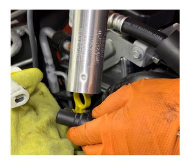
12. NOTE- we are only replacing the one upper fitting on this tube as the lower fitting is very difficult to get to.
