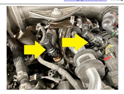
3. Locate the U shaped PCV hose and remove it by releasing the quick release fittings.
