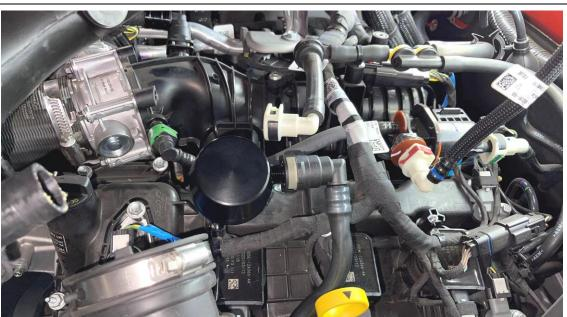
13. To install the Clean Side Separator, (CSS) pull up on the collar at the base of the CSS and push it down onto the CCV fitting on the valve cover. Once the CSS is installed fully onto the CCV fitting, the collar will click on to secure it. A little oil applied to the valve cover fitting can help the CSS to pop on smoothly. Rotate the fitting on the CCV tube and click it onto the CSS fitting. Reinstall the air inlet tube and ensure all fittings are connected properly.
