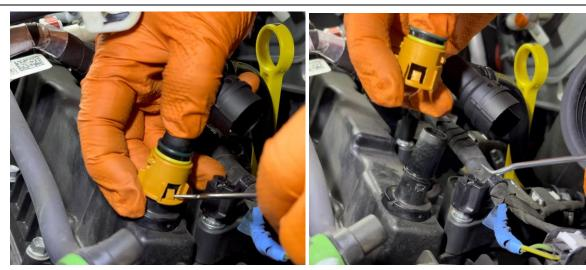
11. Once the outer cover of the fitting is off, while applying upward pressure, use a pick or small screwdriver to release the 3 tabs and remove it.
