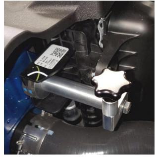
Locate the factory PCV / vacuum fitting. On some Mid '21 and all '22 Rangers it wil be on the top of the intake manifold next to the EVAP solenoid on the driver side of the engine. To release the fitting, press the button on the fitting and lift it off of the intake manifold. (As pictured, the button will be *under* the fitting. You should never pry or remove the button)
