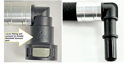
5. Connect the dirty side of the catch can system by twisting the fitting in the factory hose to make it easier to connect to the UPR male connector on the PCV hose. Then, connect the '12.61' Female fitting to the Intake Manifold vacuum port.
