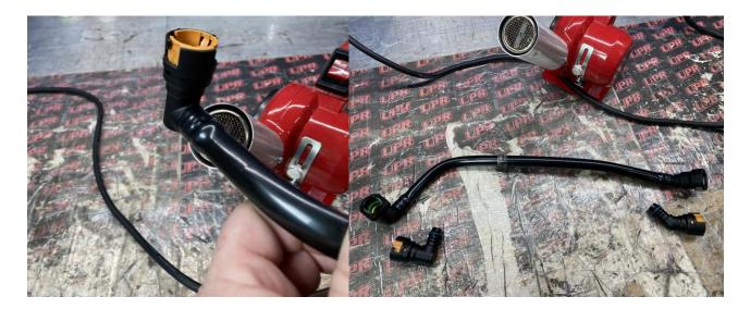
7. To install the Clean Side Separator (CSS) pull up on the collar at the base of the CSS and push it down onto the CCV fitting on the valve cover. Once the CSS is installed fully onto the CCV fitting, the collar will click on to secure it.
