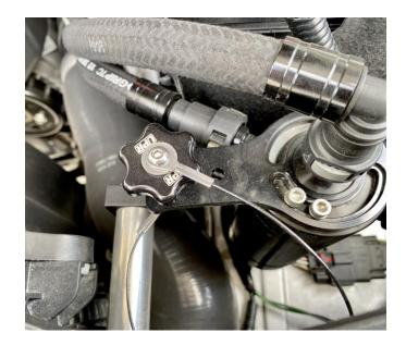
3. The Wide Open Throttle Hose will connect from the 90 Degree fitting on the catch can, and route along the fan shroud towards the Turbo intake tube. Be sure the arrow on the check valve is facing away from the catch can.
