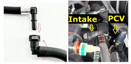
6. Route the hoses towards the UPR catch can and connect them as shown. PCV to the top of the catch can, Intake manifold vacuum to the side of the catch can.
