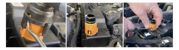
Now that you can see the 3 tangs, while applying upward pressure, use a pick or small screwdriver to release them and remove the rest of the fitting from the valve cover. Repeat the process on the fitting at the other end of the hose at the turbo inlet tube.
