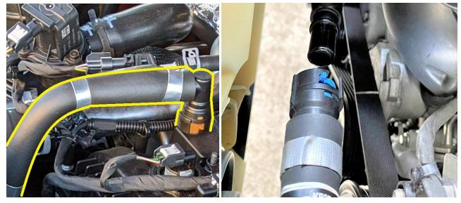
Follow the tube to the end where it connects to the turbo inlet and release the fitting (most will have a tamper Proof fitting at both ends instead of the quick release fittings).
