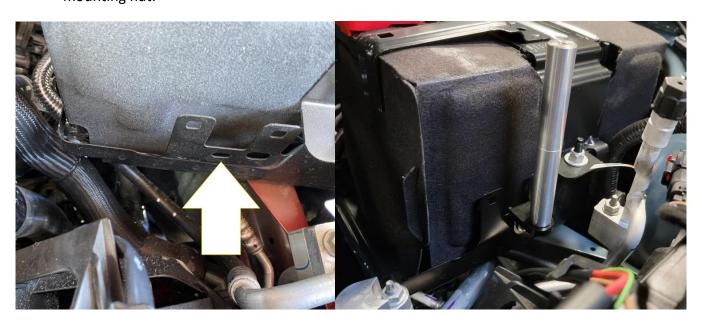
2. Fasten the catch can onto the bracket and tighten the UPR quick release knob (Style May vary from photo). You can 'clock' the position of the catch can by loosening the allen screws on top for optimal positioning.
