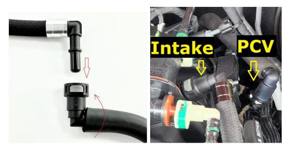
6. Route the hoses towards the UPR catch can and connect them as shown. PCV to the top of the catch can, Intake manifold vacuum to the side.
