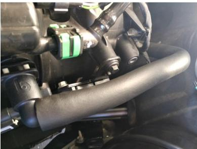
4. The catch can hoses will have a special '12.61' female fitting for the intake manifold vacuum fitting, and a Male 90 Degree fitting for the 'Dirty' or PCV side which will connect to the factory PCV hose.
