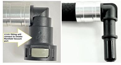
5. Connect the dirty side of the catch can system by twisting the fitting in the factory hose to make it easier to connect to the UPR male connector on the PCV hose. Then, connect the '12.61' Female fitting to the Intake Manifold vacuum port.
