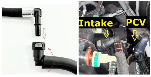
6. Route the hoses towards the UPR catch can and connect them as shown. PCV to the top of the catch can, Intake manifold vacuum to the side of the catch can.
