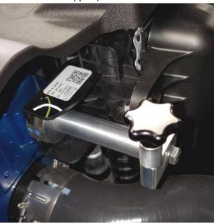
2. Locate the factory PCV / vacuum fitting. On some Mid '21 and all '22 Rangers it wil be on the top of the intake manifold next to the EVAP solenoid on the driver side of the engine. To release the fitting, press the button on the fitting and lift it off of the intake manifold. (As pictured, the button will be *under* the fitting. **You should never pry or remove the button**)
