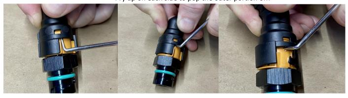
Now that you can see the 3 tangs, while applying upward pressure, use a pick or small screwdriver to release them.
