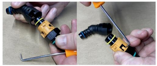
To replace the fittings on your factory CCV tube, use a heat gun or lighter to gently warm the plastic tube – do not melt or burn the tube. Pull the fitting out of the tube once it is warm, and insert the new fitting into the tube while it is still warm. The tube will conform to the fitting as it cools. To assist, you can wrap a small zip tie around the tube ends while it cools.
