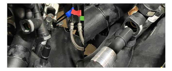
Remove the 10MM nut on the ABS brake controller bracket. Install the UPR Clean Side Catch Can bracket and reinstall the nut. You may bend the bracket slightly to allow the catch can to sit level.
