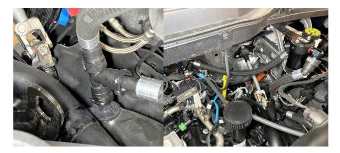
Go back through and check all connections. Check the catch can about every 1000 miles until you get a good feel for what your engine will expel. Most will need to service the catch can at oil change intervals.
