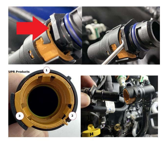
Once the CCV fitting is removed from the valve cover, You can rotate it to get a better view. Use a 90 degree pick to depress the 3 tangs on the orange fitting. While depressing the tangs, you will need to apply light outward pressure to the CCV fitting as if you are trying to pull it out. This way, once the tangs are pressed the fitting can come out.
