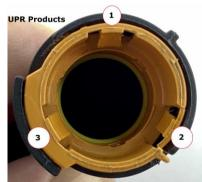
While holding the hose and applying slight upward pressure, run the pick under the fitting to release the tabs. If the fitting or tabs break, the fitting can be replaced with a standard UPR Plug and Play fittings P/N 2025-39 (straight), 2025-40 (90 degree) or 2025-41 (45 degree). Repeat the process to remove the fitting at the other end of the tube.
