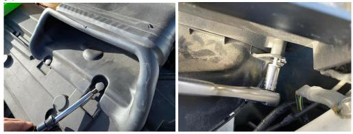
2. Locate the oval shaped hole in the frame on the driver side directly below the air inlet. Install the 90 degree mounting bracket to the frame with the supplied hardware. The bracket should be facing upwards as shown. Install the catch can onto the bracket with the supplied hardware.
