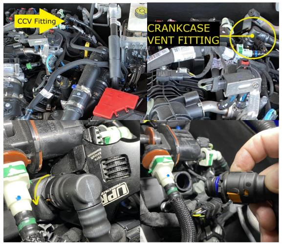
The female orange fitting does not have a quick release mechanism. To remove it, use an adjustable wrench or 1 1/16" claw foot wrench to turn the CCV fitting on the valve cover counter clockwise about ½ turn and lift it off.
