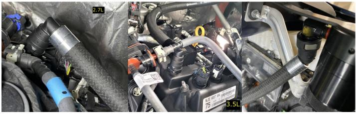
Install the shorter hose that has 45 degree fittings onto the front fitting on the clean side catch can, then connect it to the male fitting on the 3 Way Tee.
