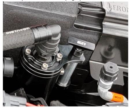
2. Attach the catch can to the UPR billet bracket with the supplied knob. You can leave the catch can slightly loose to allow adjustment when routing hoses. The allen screws at the top of the catch can allow for adjustment as well. Once the hoses are routed, adjust the catch can for best fit and tighten fasteners.
