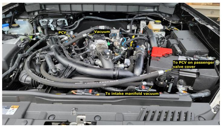
4. Connect the hose with 45 degree fittings from the side of the catch can to the intake manifold vacuum port. Connect the hose with 90 degree fittings from the PCV valve on the passenger valve cover to the top of the catch can. You can secure the hoses if desired with zip ties, but if routed as shown they will be secure.
