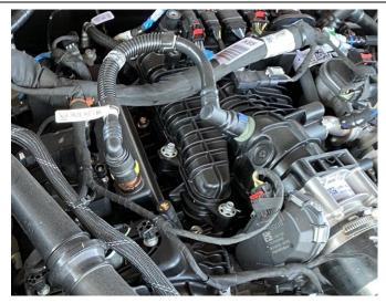
3. Locate the U shaped PCV hose and remove it by releasing the quick release fittings. Save this hose in case you ever want to return the vehicle back to stock.
