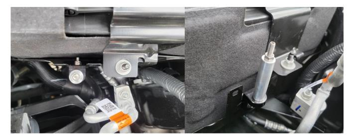
1. Using the supplied hardware, attach the UPR billet catch can mounting bracket to the middle hole at the front of the battery tray. To make this easier, you can remove the battery hold down bracket which will allow you to move the battery slightly.
