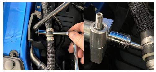
2. Install the UPR catch can using the supplied quick release knob.
