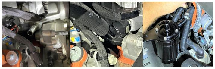
5. The 'Dirty Side' Hose will have 90 degree fittings on both ends. Connect one end to the valve cover fitting, and the other to the top fitting on the catch can.
