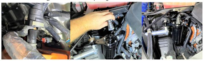
Always check and drain the catch can more often in winter / freezing weather. If the water/oil mixture in the catch can is allowed to freeze it will cause damage to the catch can and internal components. Any damage due to freezing is NOT WARRANTY. You must dispose of the liquid collected in the catch can properly (with used waste oil) properly according to your local laws.
